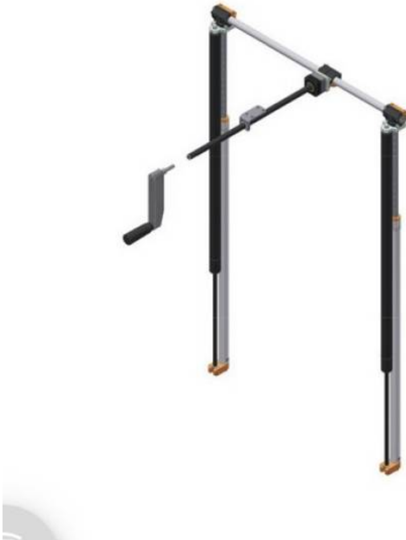
Figure 20: Crank lifting system
