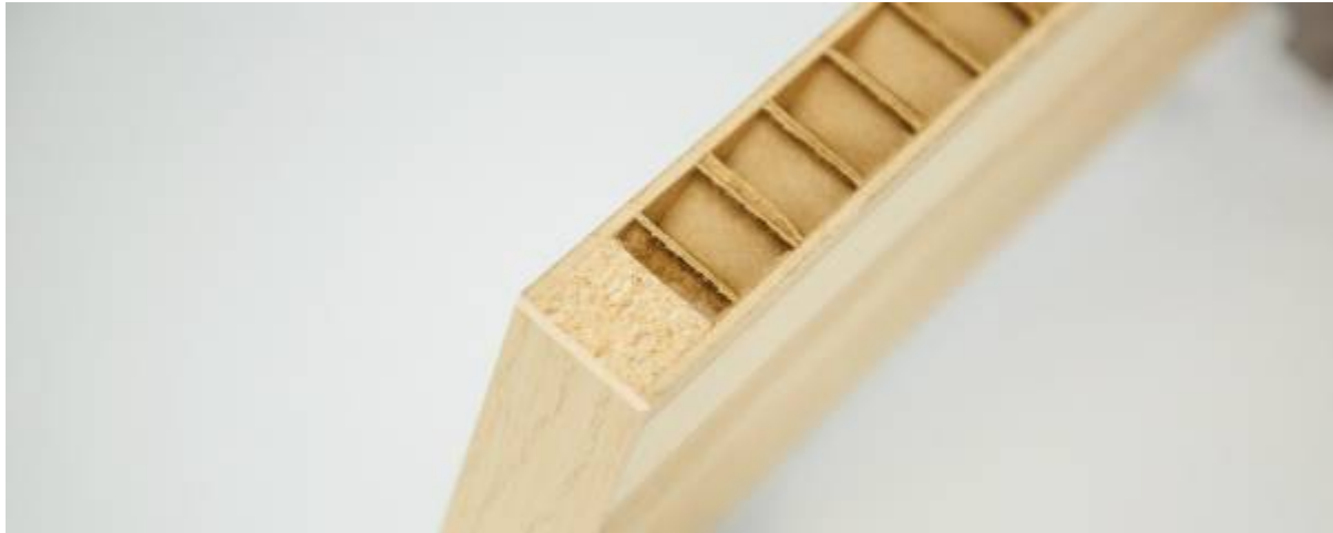
Figure 19: Composite with honeycomb core
