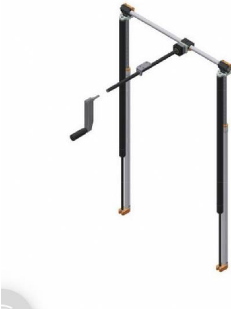
Figure 21: Crank lifting system
