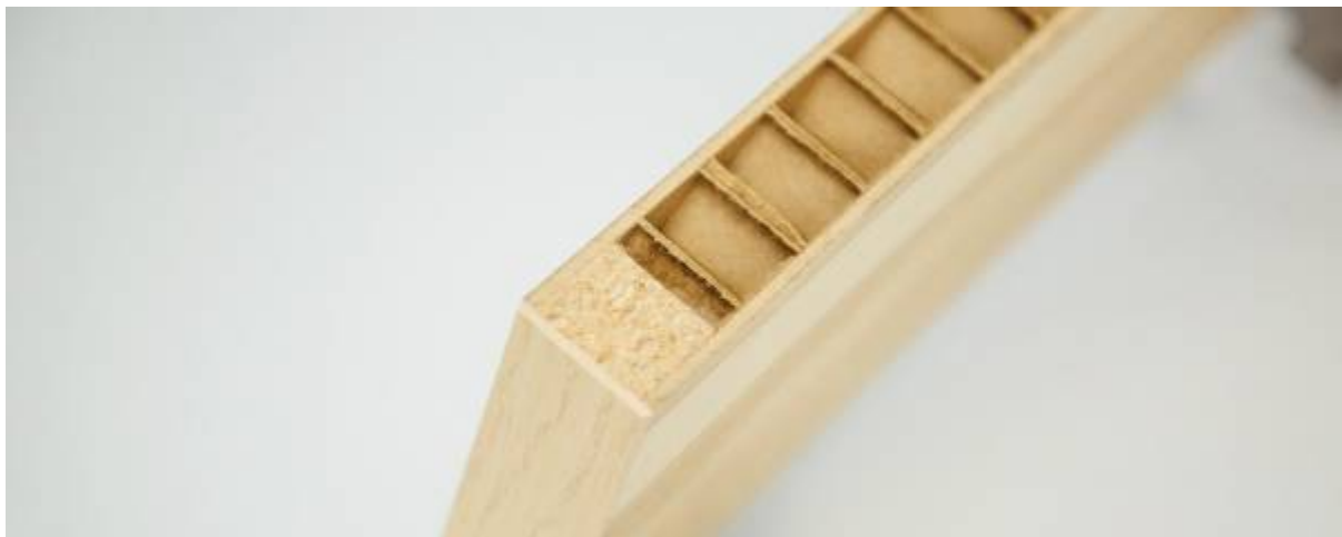
Figure 21: Composite with honeycomb core
